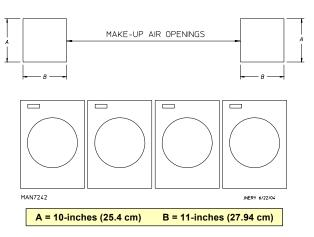
EXAMPLE: For a bank of 4 MDG31 dryers, 2 unrestricted openings measuring 10-inches by 11-inches (25.4 cm by 27.94 cm) are acceptable.
